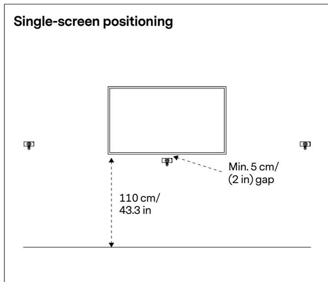
Position the side cameras at an appropriate distance from the screen to capture all participants. For the center camera, maintain a minimum 5 cm/2-inch gap from the screen.
