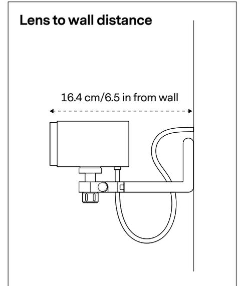
The total distance between the back wall and the front of the camera is 16.4 cm/6.5 inches.
