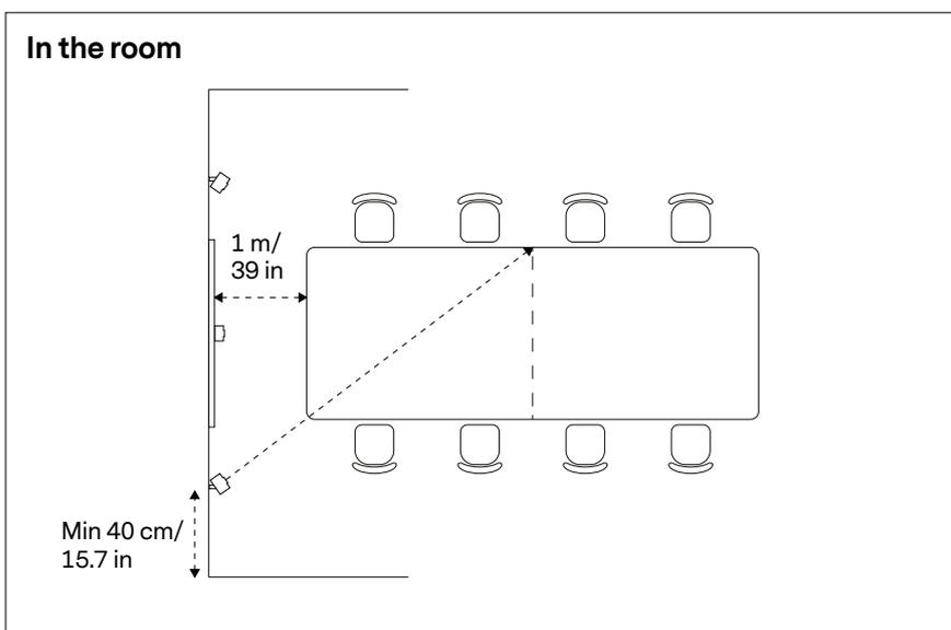
Side cameras: Keep a minimum of 40 cm/15.7 inches distance from side wall to bracket center. Angle them diagonally towards the table's center. Center camera: Place it at least 1 m away from the table.
