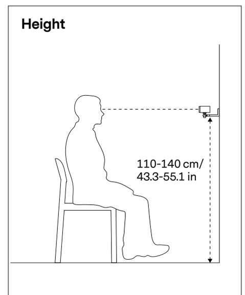
Place cameras at eye level to enable eye contact between remote and in-room participants.
